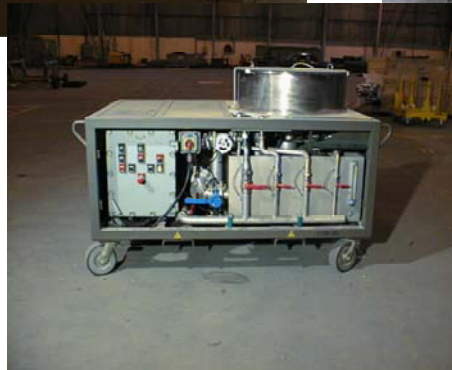
Figure 6-45: I Level Ground Test Utilities for Trouble Shooting.
