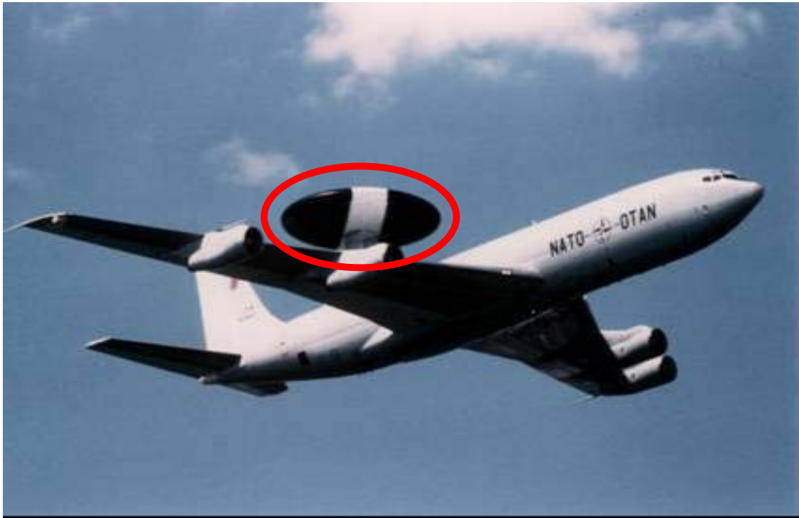
Figure 6-16: AWACS E3A Aircraft – Detection of Debonds in ROTODOME Structure.
