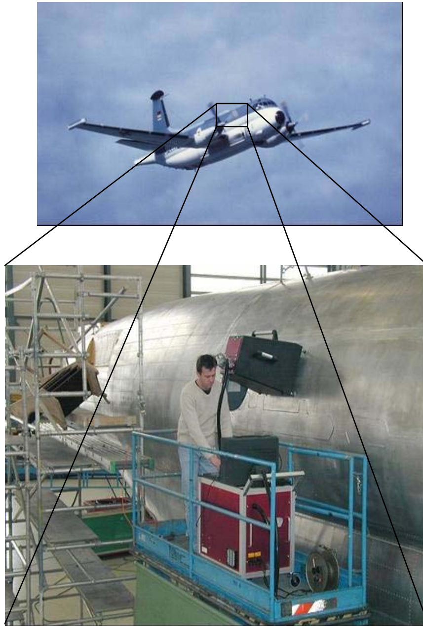
Figure 6-19: Breguet Atlantic Aircraft – Detection of Debonding in Honeycomb Structure in the Fuselage and Wing.
