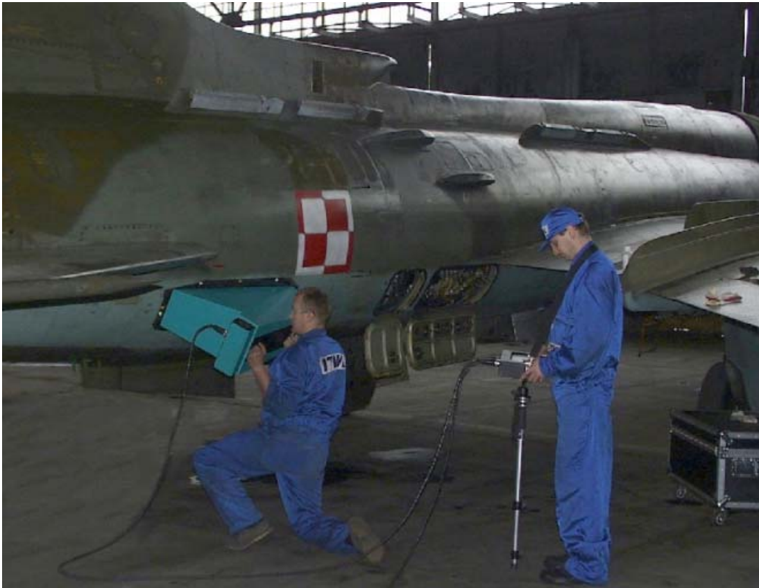
Figure 3-5: The DAIS System in Operation.
