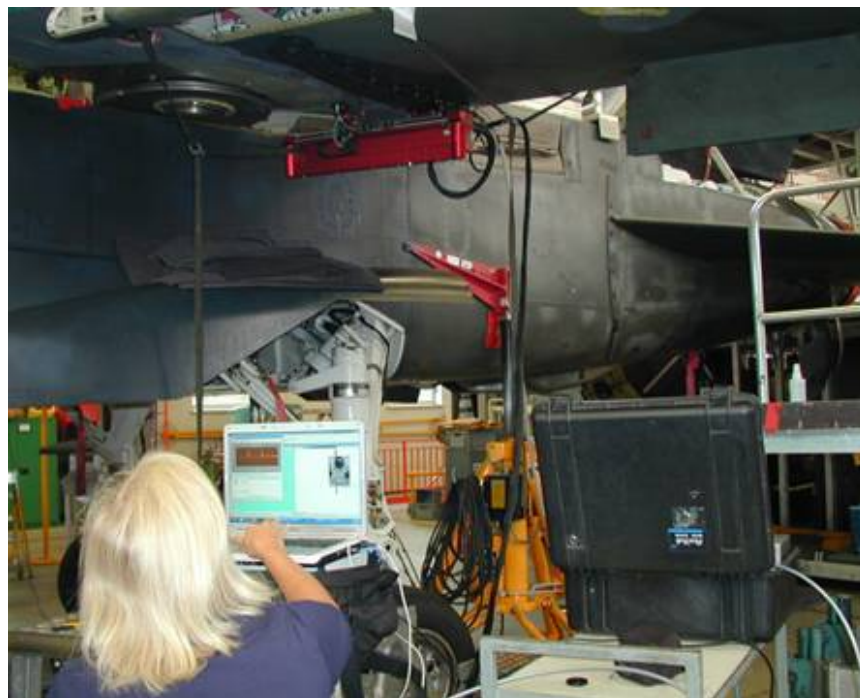
Figure 6-18: Tornado Aircraft – Detection of Corrosion at the Wing Diffusion Joint.
