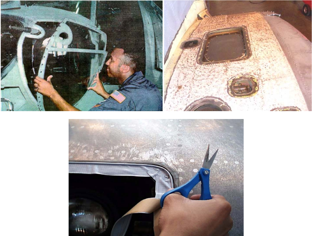
Figure 6-97: Skyflex Aircraft Sealant – “Peel and Stick” Teflon Foam Tape Substitute for 2-Part Paste Sealants.
