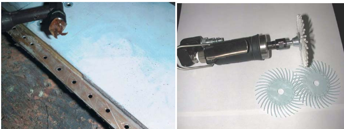
Figure 6-98: Bristle Discs and Rotary Cutters from 3M Simplify and Speed Sealant Removal and Reduce Solvent Use.
